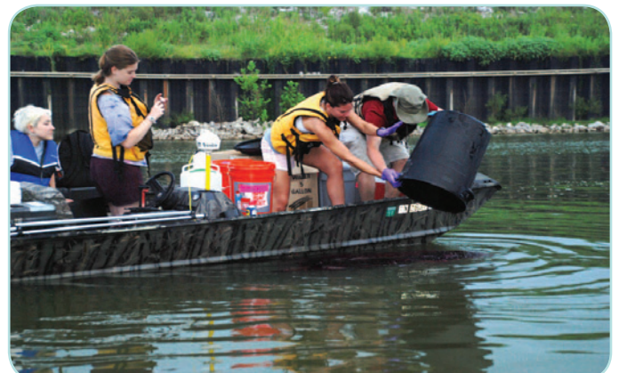
AAT field crew releasing dye for time-of-travel
