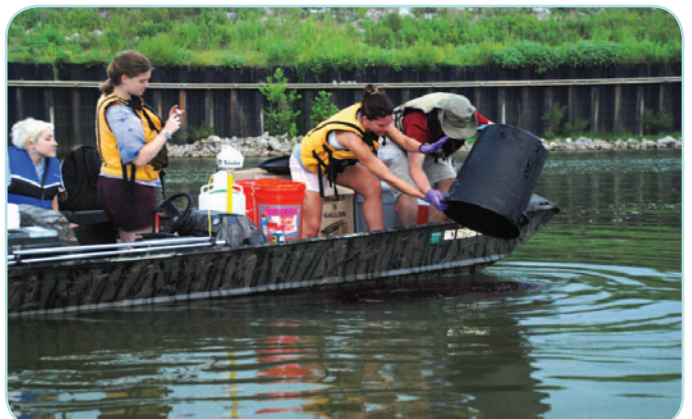
AAT field crew releasing dye for time-of-travel
