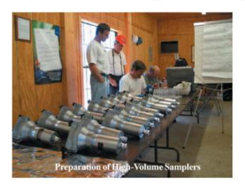
and low-flow rate sampler was calibrated prior to the test and at the test's conclusion. This project required 16 high-volume air samplers for PAHs, metals, and dioxins/furans; over 40 negative-pressure sample vessels for VOCs; and over 30 low-volume air sampling pumps for phenolics. All of the sampling media cartridges were prepared along with duplicates, blanks, and spiked samples for laboratory and field quality control purposes. Three remaining team members arrived one day prior
