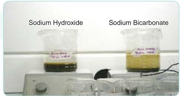
Figure 1. Caustic vs. Bicarbonate Precipitate
